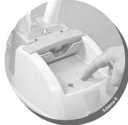
If you wish to stop the robot during the cycle, press the OFF button. **Figure 7**.
